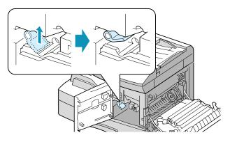
4 Remove the drum cartridge from its bag and slide it into the product firmly until it locks into place completely.
